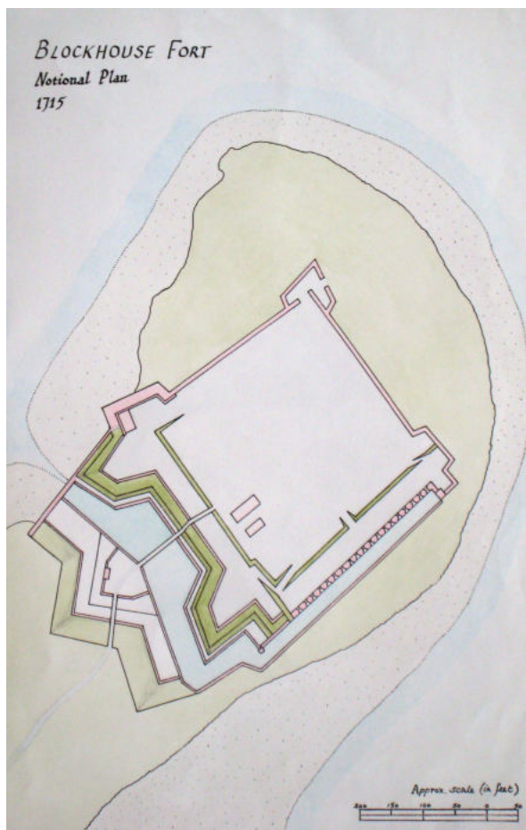
Figure 20 1715; the fort as rebuilt during Queen Anne's time. Of particular interest here, the outer wall at the bottom of the plan approximates to the position of the 2013 damage; a notional plan adapted from some two dozen partial or low quality images, viewed at multiple places. CHD.
