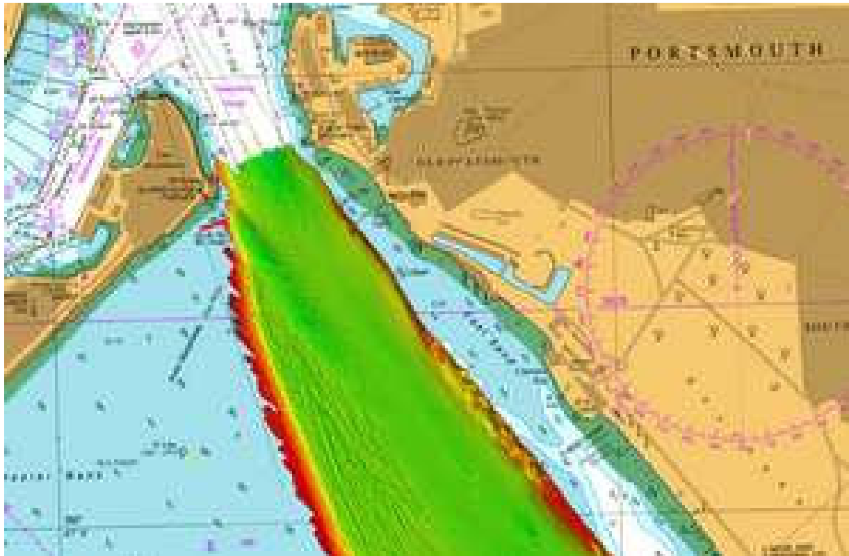
Figure 36 Bathymetric Data for Portsmouth approaches gathered by HMS Gleaner , showing the actual profile, post-dredge. Hamilton Bank is immediately to the south of the Fort, to the right of Haslar Bank; the red colour represents near vertical sides; UK Hydrographic Office, published Aug 2017 [i.e. post-dredge]. © UKHO.
