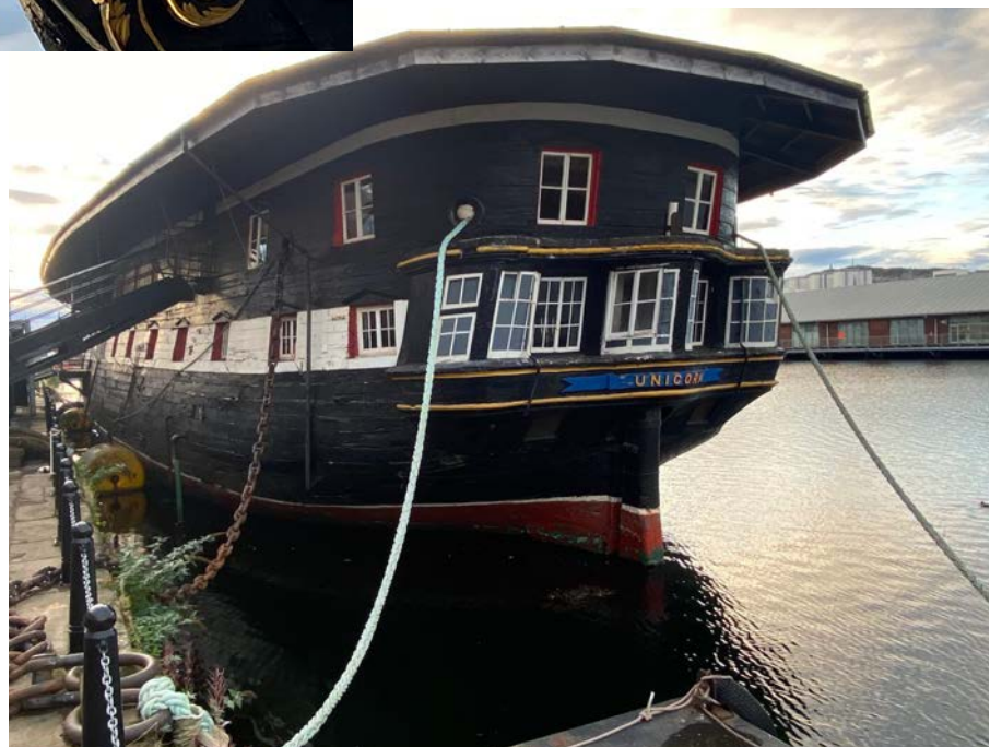
Right: HMS Unicorn : Sir Robert Seppings' elliptical stern.
